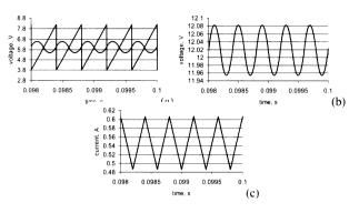
Fig. 2. The nominal period-1 operation of the buck converter: (a) the control and ramp signals, (b) the output voltage, and (c) the output current. The parameter values are  $V_{\rm in} = 24V$ ,  $V_{\rm ref} = 11.3V$ , L = 20mH,  $R = 22\Omega$ ,  $C = 47\mu F$ , A = 8.4, T = 1/2500s, the ramp signal varies from 3.8V to 8.2V.
