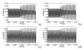
Fig. 6. System output voltage and current time response shows period-1 behavior which is gone to unstable period-2 at time 0.105 with, (a) original model (b) TS fuzzy model. Likewise the current time responses with (c) original model (d) TS fuzzy model.
