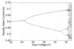
Fig. 7. Bifurcation diagram of the TS fuzzy model of buck converter varying input voltage as a parameter.
