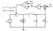
Fig. 1. The voltage mode controlled buck dc-dc converter.
