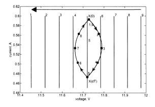
Fig. 3. Period 1 limit cycle, the 9 different points indicate the location of the time varying switching surface at theses instants.
